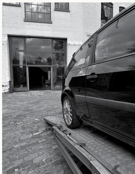
The cars were engineered to be liftable by hi-ab crane truck or transported by conventional flatbed breakdown vehicles. ©David Cotterrell
